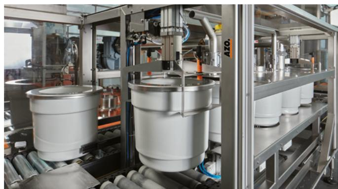
Target containers are placed into the dosing line
