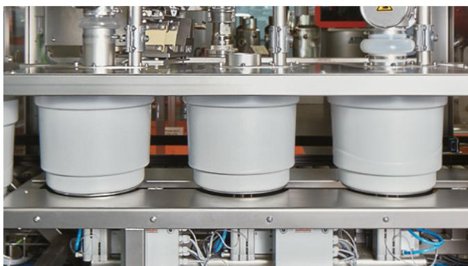
Individual scales enables simultaneous weighing
