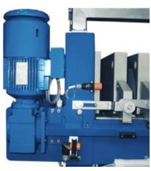
Optional vibrating device for faster filter cake discharge and thus shorter cycle times
