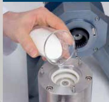
*Filling with the grinding beads is easy to carry out by dismantling the grinding chamber and opening the front lid*
