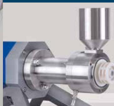
*Emptying the grinding beads and cleaning of the grinding chamber is easy to do when the grinding container is dismantled*
