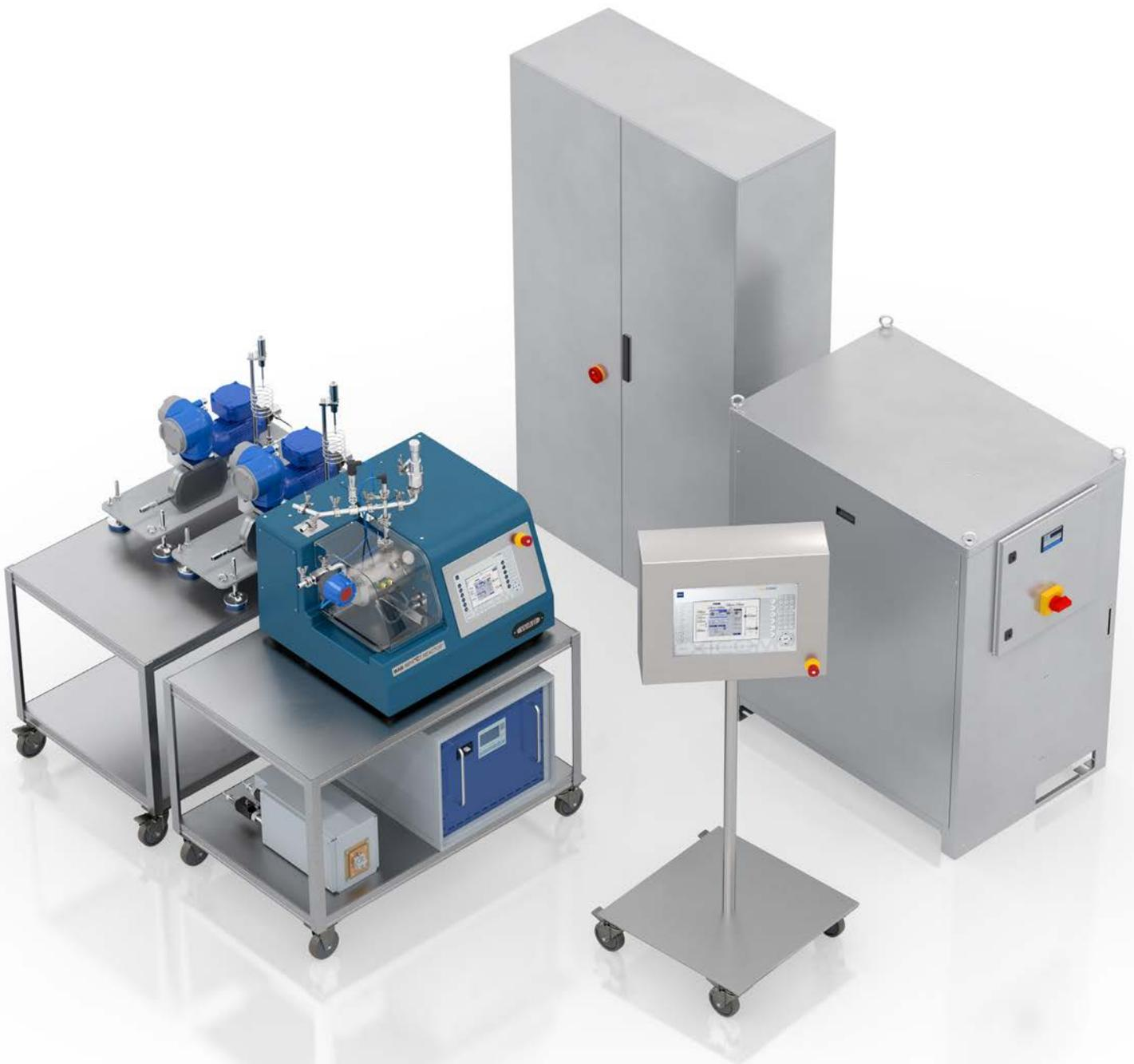
The system allows working in both passage and circulation processes. Processing starts with 1 litre of suspension and can be scaled-up to the larger models of the DYNO®-MILL series.
