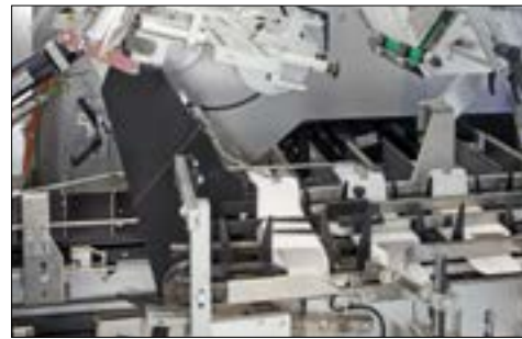
Product feed into the open cartons
