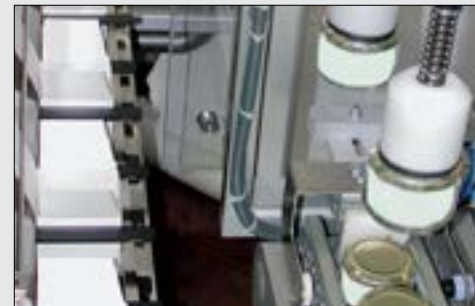
Vial feeding in intermittent mode
