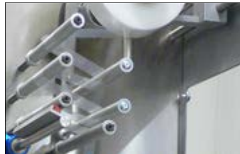
Strain release during foil unwinding
