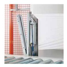
Motor-driven brush attached to pallet rollerway for perfect adherence of following edge and to prevent "fishtail" effect.
