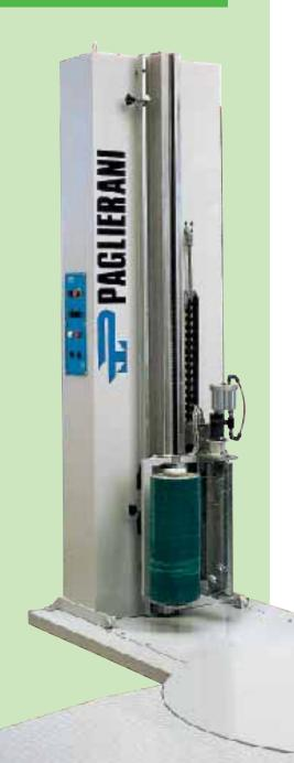
With the AV 350, the increase of the wrapping automation with a small investment is obtained. The AV 350 can be positioned in line at the outfeed of an automatic palletiser, and is suitable for low and medium speeds.
