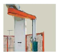
Reel holder supported by rotating arm, designed for simple and fast replacement.
