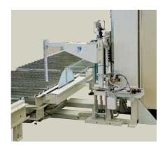
• Programmable controller (PLC) for machine control and integration with upstream equipment (palletiser).
