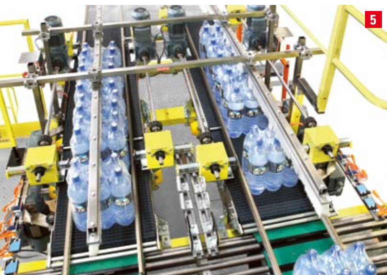
Figure 5 Two, dual-belt infeeds with motorised, automatically adjustable lateral guides
