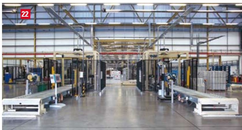
Figure 21 Laser-guided shuttle for pallet pick up and deposit to and from the palletising and depalletising lines.
