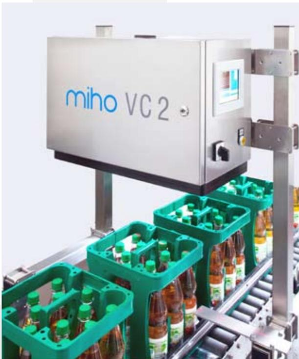
The crate inspection system **miho VC 2** inspects bottle crates after the packer to see if all bottles are present and that the trays are fully packed. It is especially distinguished by a performance spectrum not yet known concerning, for example, different crates and bottle-types.
