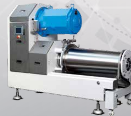
FINE GRINDING FM BALL MILL UP TO 2000 KG LIQUOR/H
